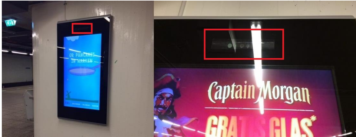
Figure 3. A digital signage panel installed at Amsterdam Central Station. On the left side is a standard advertising billboard, which is simply a TV screen and shows varying video advertisements (that is why on the left image there is a blue-colored advertisement and on the right side a red-colored advertisement even though it is the same advertising billboard). On the right side, it is a zoom-in picture of an Xbox Kinect sensor, with an assumed function of tracking the passersby (i.e., with AFRS capabilities). Xbox Kinect sensor is marked with a red rectangle. Picture taken: April 2015 by the first author.
