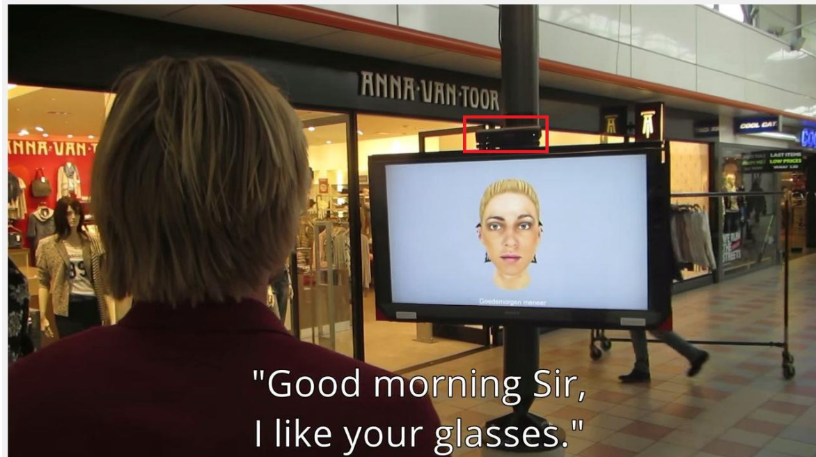
Figure 4. Real-life user interaction with a virtual shopping assistant in a commercial center in the Netherlands. It is a standard TV screen with an Xbox Kinect (with AFRS) installed on top of it. On the Figure, the AFRS is marked with a red rectangle. The avatar is able to recognize that in front of it stands a) a man and b) that he is wearing a pair of glasses. The avatar greets the person with the text visible above. Reproduced with permission.
