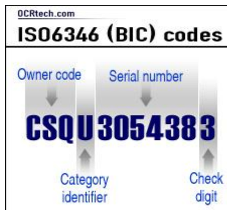
Figure 10: BIC codes, ISO 6346 - ocrtech.com
