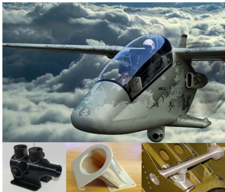
Figure 17: Locally produced AHRLAC aircraft with some components produced by AM technology
