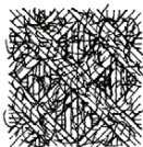
Bidirectional complex mat weave + random fibre orientation
