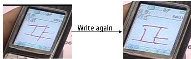
Fig. 6. The user has to rewrite the Chinese characters carefully since some strokes he input earlier were deformed
