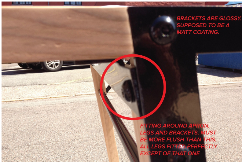
Detail of the corrections to the first piece produced
