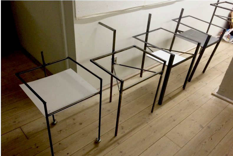
Full-scale prototypes of different versions of the trolley
