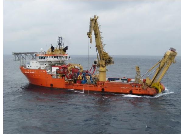
Solstad's Normand Pioneer is a pipe laying, multi-purpose CSV with several winches and cranes. Source: Solstad.no
