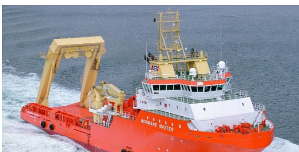
Solstad's AHTS-vessel Normand Master fitted with a 250 MT bollard pull and a 23 330 BHP engine. Source: Solstad.no
