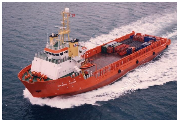
Solstad's Normand Carrier - A typical PSV-vessel at 4560 DWT and approximately 950m 2 loading space.
