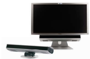
Figure 1 - SMI RED250 VOG recording systems
