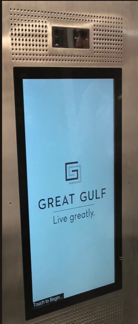
Mircom's building user interface system for Great Gulf homes
