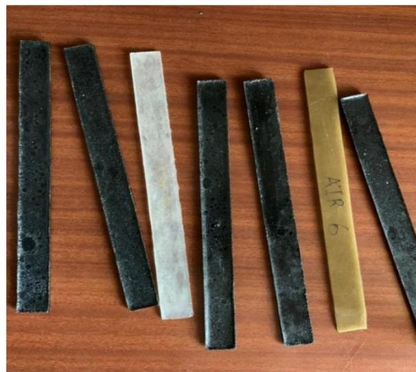
**Figure 2.** Specimens used for tensile test.
